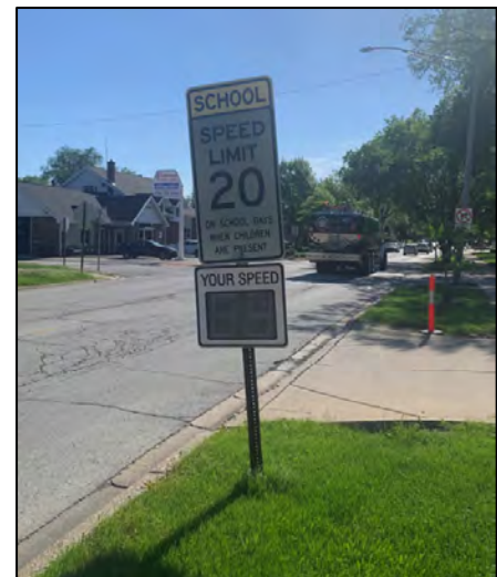
Figure 5-14. Re-locatable speed feedback sign
