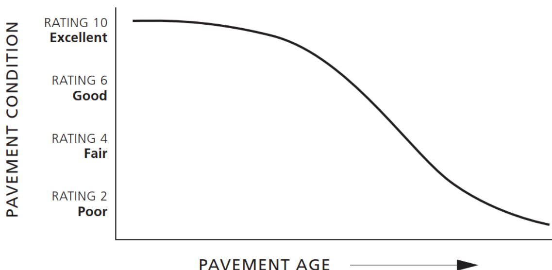
Figure 1. Pavement condition depreciation versus pavement age.
